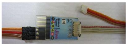
The telemetry cable has three plugs, the smallest one will not be used. This cable is identical to that which **Unilog** uses, here the small plug in addition is connected to **Unilog**, but is left unconnected with *JLog2*.
